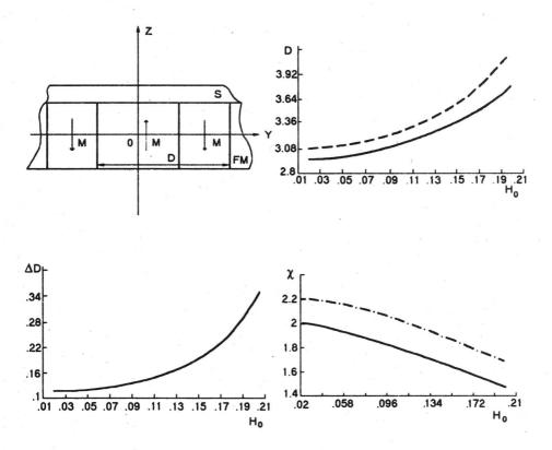
Fig. 1. The two-layer structure: S — superconductive film; FM — ferromagnetic film
