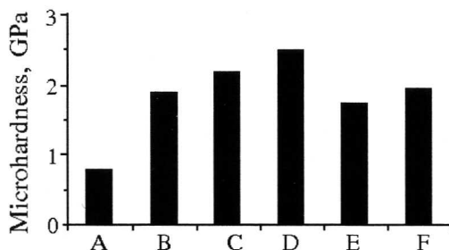
Fig. 1. Microhardness of Al–Cu–Mg-alloy 2024 after different routes of thermal treatment and severe plastic deformation (SPD): A – quenching, B – SPD at 20°C of hot-pressed state, C – SPD at 20°C of quenched state, D – regime C + natural aging, E – SPD at 200°C of quenched state, F – SPD at 20°C of quenched and pre-aged state
