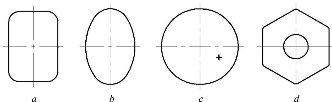
**Fig. 2.** A few examples of cross-sections of dies for twist extrusion: *a* – rectangular; *b* – elliptical; *c* – circular, ‘+’ denotes the position of extrusion axis; *d* – hexagonal with a hollow centre
