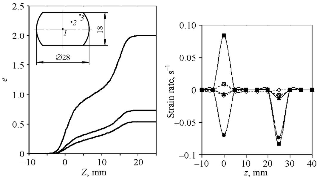
**Fig. 4.** Accumulation of von Mises strain for three typical points of the cross section (see insertions) during TE
