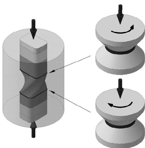
**Fig. 1.** TE scheme. The analogy of TE with HPT process was shown on the insertions
