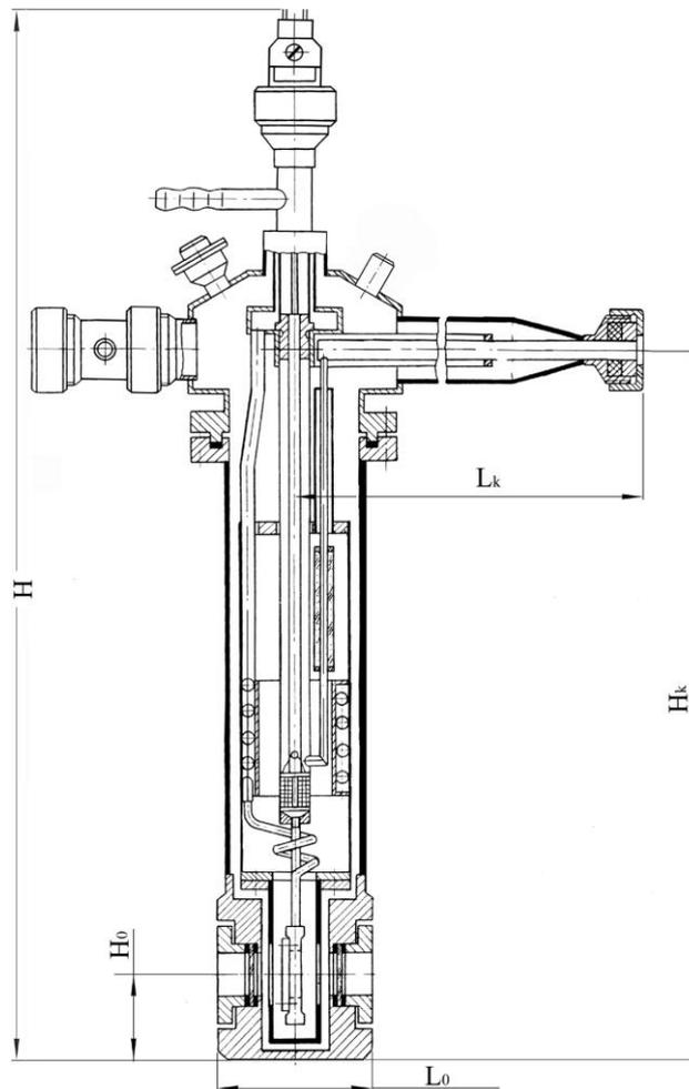
The change of standard is produced by dismantling of cryostat. For the change of standard lower parts of casing and screen are taken off.
