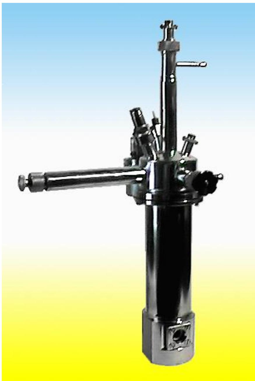
Small cryostat CT- PR is intended for research of characteristics of photosensitive materials, photoreceivers and emitters in the range of temperatures of 3-300K or 80-300K in the visible and infra-red region of radiation spectrum.
