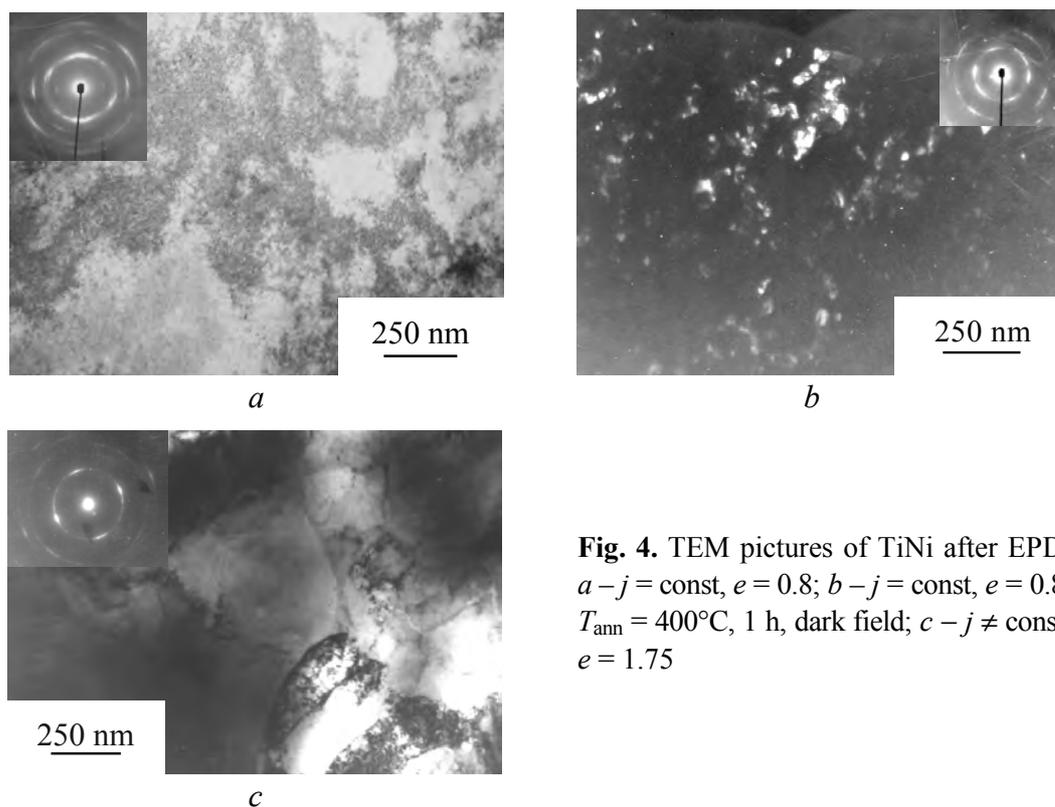
**Fig. 4.** TEM pictures of TiNi after EPD:  $a - j = \text{const}, e = 0.8$ ;  $b - j = \text{const}, e = 0.8, T_{\text{ann}} = 400^\circ\text{C}, 1 \text{ h}$ , dark field;  $c - j \neq \text{const}, e = 1.75$
