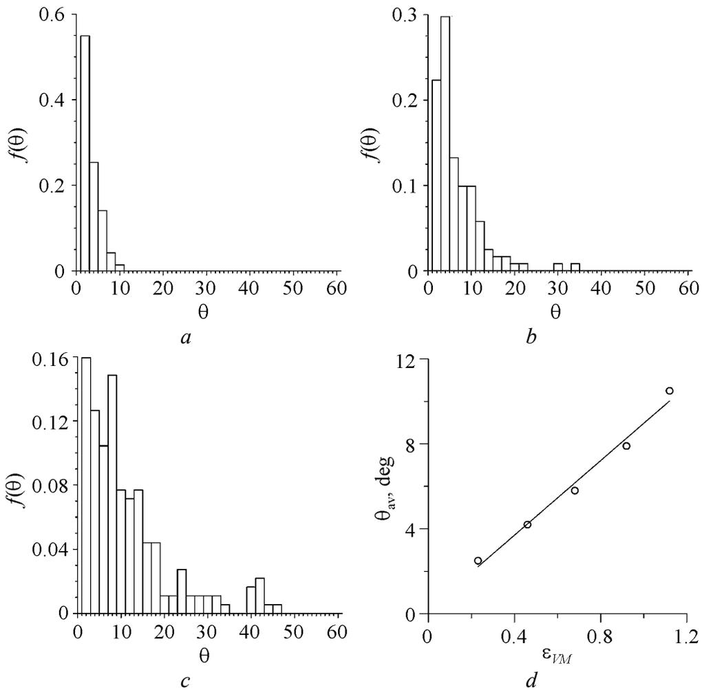
**Fig. 2.** Evolution of the conditional misorientation distribution function during simple shear strain up to  $E_{VM} = 0.23$  (a), 0.68 (b), and 1.12 (c) and a plot of the average misorientation angle of subgrains with strain (d)
