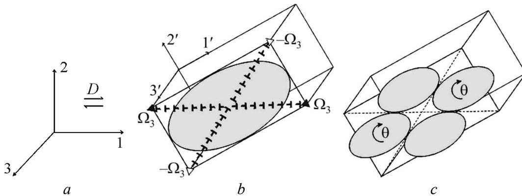
**Fig. 1.** A model of grain subdivision by a growth of a pair of subboundaries along the grain diagonals: *a* – coordinate frame: 1 – shear direction, 2 – normal direction, 3 – transverse direction; *b* – a junction disclination quadrupole and a mode of its relaxation; *c* – new grains (subgrains) formed due to subdivision
