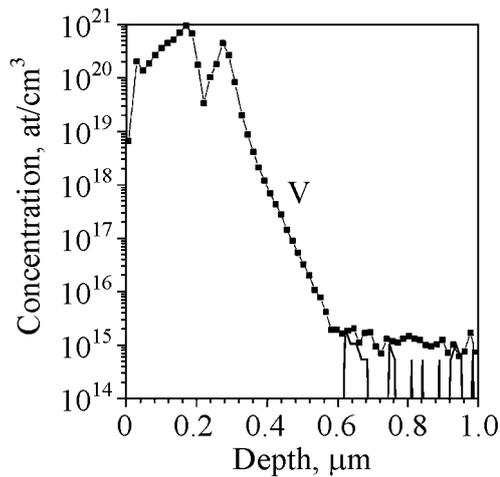
**Fig. 5.** SIMS depth profile of V in Si:V processed for 5 h at 1270 K under 1.1 GPa
